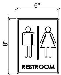
BRAILLE RESTROOM SIGN
